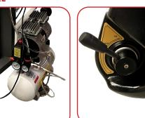
The movement of the upper roller is controlled by a compressor, supplied with the machine. It is very simple to operate with an easily accessible lever for an opening up to 45mm.
